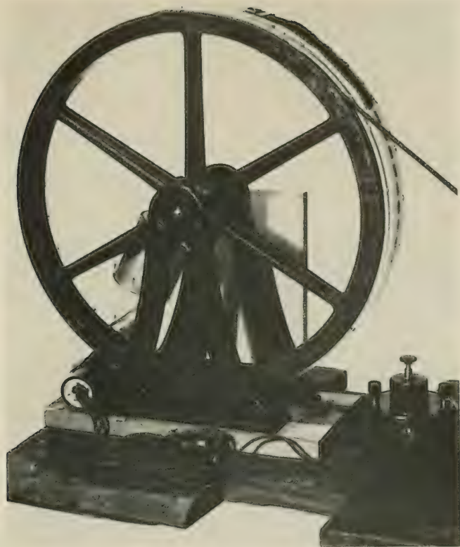
1. PHOTOELECTRIC APPARATUS FOR ANALYSIS OF TRANSIENT SOUNDS.
