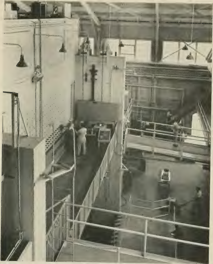
Preparing to remove plugs from some of the 1,248 fuel-channel openings in the shield of the Oak Ridge graphite reactor, personnel stand on an elevating platform. In brackets on the wall of the elevator, in front of the two men, can be seen a horizontal bundle of 10-foot lengths of light steel poles used as "push rods." As a rod is inserted into a channel, another rod is threaded to it, increasing its length to permit traversing the length of the fuel channel.
